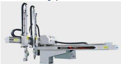
BRB600/700 Series is applicable to all types of horizontal injection machine ranges of 60~200T for take-out products and sprues. Vertical arm is single type, with product arm and runner arm two types, suitable for two plate or three plate mold products take out. Traverse axis driven by AC servo motor. After installed this robot, the productivity will be increased 10~30%, reduce defective rate, ensure safety operators, reduce manpower and accurately control the output to reduce waste.
